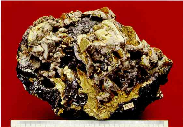
埼玉県秩父鉱山の閃亜鉛鉱・黄銅鉱・石英 Sphalerite, chalcopyrite and quartz, Chichibu mine, Saitama
